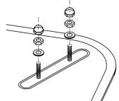
Do not tighten the screws before adjustment.
